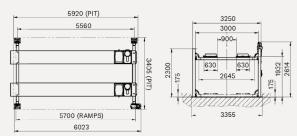
**4500.3IMOT7** - Five tonne Class 7 ATL/OPTL four post electro-hydraulic lift.
